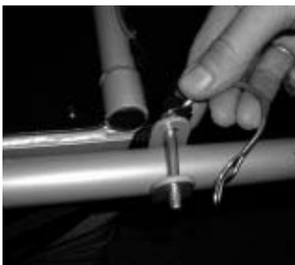
Push the longer spring clip bolt through the hole in the U-shaped socket and secure it by locking the spring clip.
