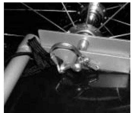
Lock the bolt by moving over the spring clip. The spring clip loop must enclose the bolt after locking.
