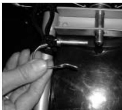
Push the spring clip bolt through the hole in the axle.
