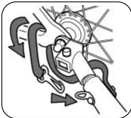
Secure the drawbar by putting the safety tie around the rear section of the bicycle frame and fastening it to the drawbar ring with the snap hook.
