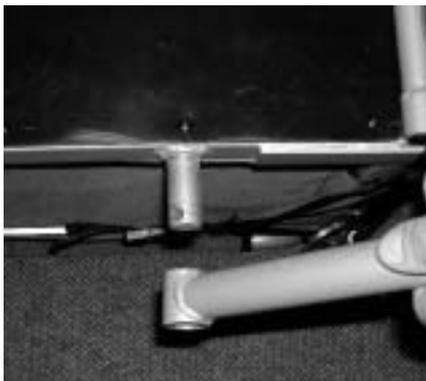
Guide the drawbar fitting over the drawbar spigot on the left hand side of the frame.
