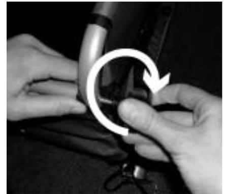
Tighten both diagonal tubes using the star grip bolts, which are attached by small ties.
