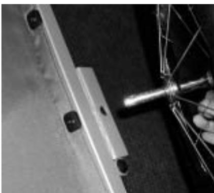
Guide the axle into the socket of the square frame.
