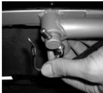
Push the shorter spring clip bolt through the hole in the drawbar spigot and secure it by locking the spring clip.
