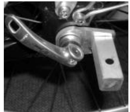
Tip: For bicycles where the length of the standard quick release is insufficient, a special quick release with longer axle is available.
