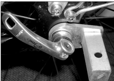
Detach the quick release and guide it through the coupling unit along with the quick release axle. Push the quick release through the hollow axle again, attach the nut and clamp the quick release with the correct prestress. At the same time align the coupling unit horizontally, along with the quick release lever, so that the square drawbar connector fits on top. (see also illustration 1 in 2.1.2.)
