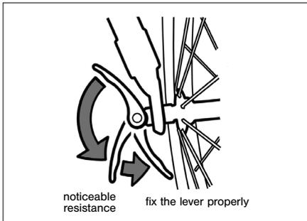
In order to ensure that the hub is clamped sufficiently in the hollow axle, the Q.R. lever must begin gripping as it moves from the open to the middle position, and approaching the closed position you should clearly feel resistance as you tighten. If it is too easy or too difficult to move the quick release lever, tighten or loosen the Q.R. lock nut on the other side of the hub.
