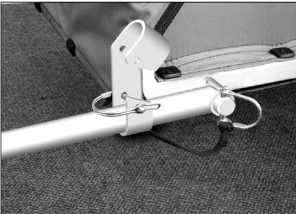
For use as a bicycle trailer engage the drawbar in the lower position in the drawbar yoke. Push the longer spring clip bolt through both of the lower holes in the drawbar yoke and secure it by moving over the spring clip loop. After locking, the spring clip loop must surround the bolt.
