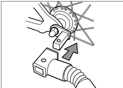
Push the square drawbar connection over the coupling unit attached to the bicycle.
