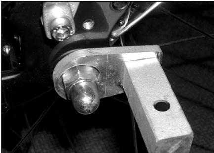
Remove the left hand axle nut. Any spacers or plain washers can generally be retained. Put the coupling unit on the axle and reattach the nut. Hold the coupling unit horizontal throughout.
