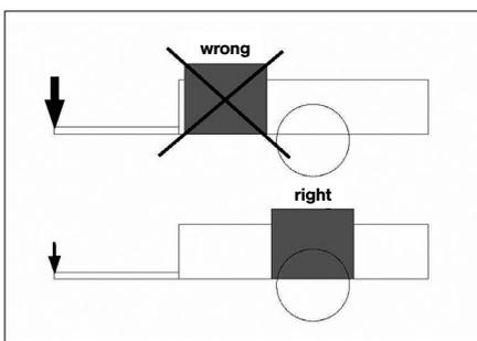
The handling of a bicycle trailer very much depends on how the load is distributed in the trailer. Too much weight in front of the wheel axles of the trailer increases the nose weight at the coupling and makes the handling and control of the bicycle harder. For this reason always load heavier objects in the area over the wheel axles.
