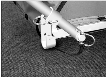
For use as a handcart engage the drawbar in the upper position in the drawbar yoke. Push the longer spring clip bolt through both of the upper holes in the drawbar yoke and secure it by moving over the spring clip loop. After locking, the spring clip loop must surround the bolt. The drawbar can be switched from the lower to the upper position without being taken off.
