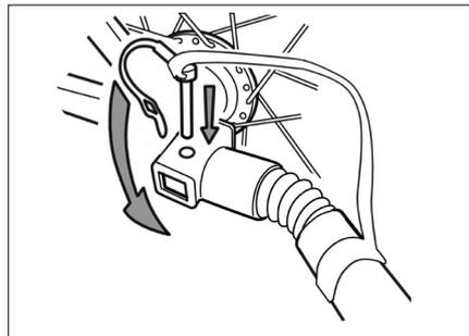
Insert the spring clip bolt through the holes of both coupling parts and close the clip so that the clip opening surrounds the bolt end.
