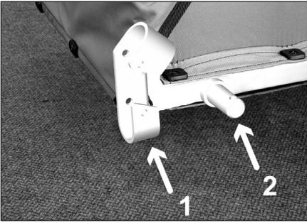
The drawbar attachment bracket of the Cargo Croozer allows you to fix the hitch arm in two positions: the lower position is for use as a bicycle trailer, the upper for use as a handcart. The drawbar attachment bracket consists of the drawbar yoke (1) and the drawbar spigot (2).
