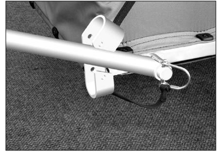
Push the drawbar as far as it will go onto the spigot. Push the shorter spring clip bolt through the hole in the drawbar spigot and secure it by moving over the spring clip loop. After locking, the spring clip loop must surround the bolt.
