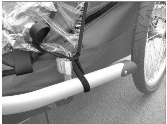
**7th step:** Pull the elasticated loop in the middle over the buggy wheel bracket.
