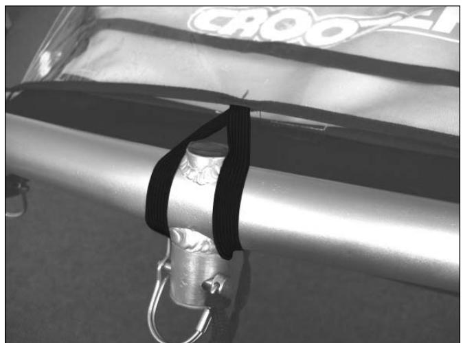
**8th step:** Fasten both sides of the rain cover to the bumper using the velcro fasteners.
